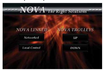
On or Networked (Mode): The Up and Down functions are enable in the programming when in the ON/Networked state. Users will now be able to control the trolleys on the control system page/menu and local UP and DOWN buttons will be disabled on all trolleys connected to the Nova Linked System (NLS).
