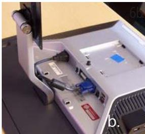
6b. Attach the video and power cables to your monitor. Allow enough slack in cables for easy tilting of monitor, but do not allow them to touch the work surface or interfere with Trolley operation
