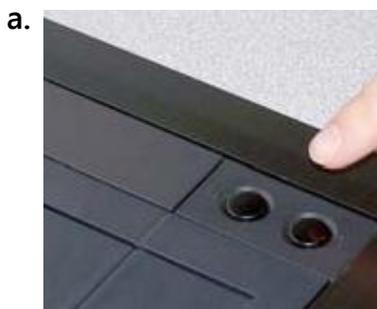
7a. Push "Down" button for a few seconds to activate unit. Once the monitor is completely lowered into the Trolley™, the door will close automatically.
