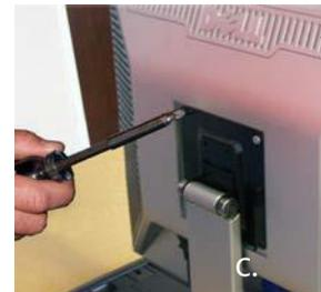
6c. Attach monitor to VESA plate using the four removed monitor screws.
